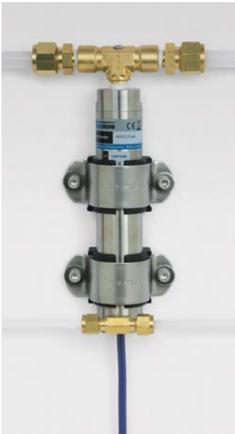
Model 4655 Multipoint Settlement System, vibrating wire pressure transducer.
