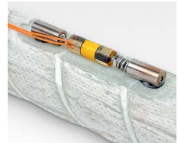
Model 4151 Strain Gauge mounted to a fiberglass rebar.
