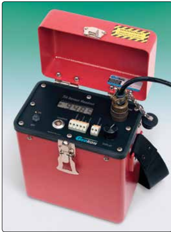
● The Model RB-500 MEMS Readout for use with the Model 6161 Tilt Sensors.
