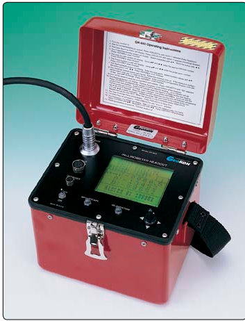
● Geokon Model GK-603 Readout Box for use with the Model 6201.
