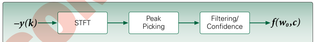
• Digital signal processing technique used to ensure correct initial measurement.
