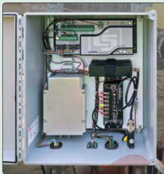
● Model 8025 Micro-800 with radio modem (configured for a Model 6150 MEMS In-Place Inclinometer).
