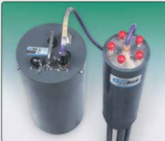
• Model 8026 Datalogger and Model 1150 (A-3) Extensometer (shown on right).
