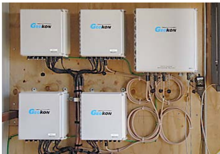
Four Model 8032 Multiplexers connected to a Model 8600-1 Datalogger.
