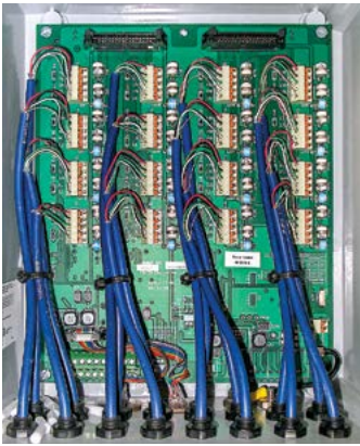
Model 8032 16 Channel Multiplexer showing internal sensor connections.*
