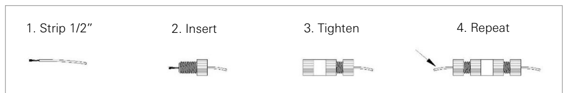
FIGURE 5: Posi-Lock Connector Guide
