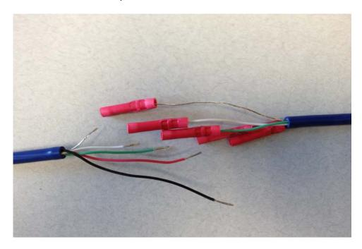
Crimp butt connectors to cable #2:
