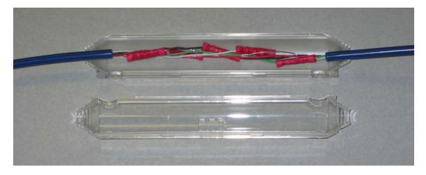
Place second mold half over the first and snap together firmly:
