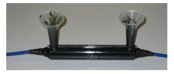
Removing the poring spouts after the epoxy has cured completes the splice:
