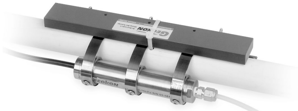
Figure 10 - 4500MLP zip Tied for Drop Weight Method
