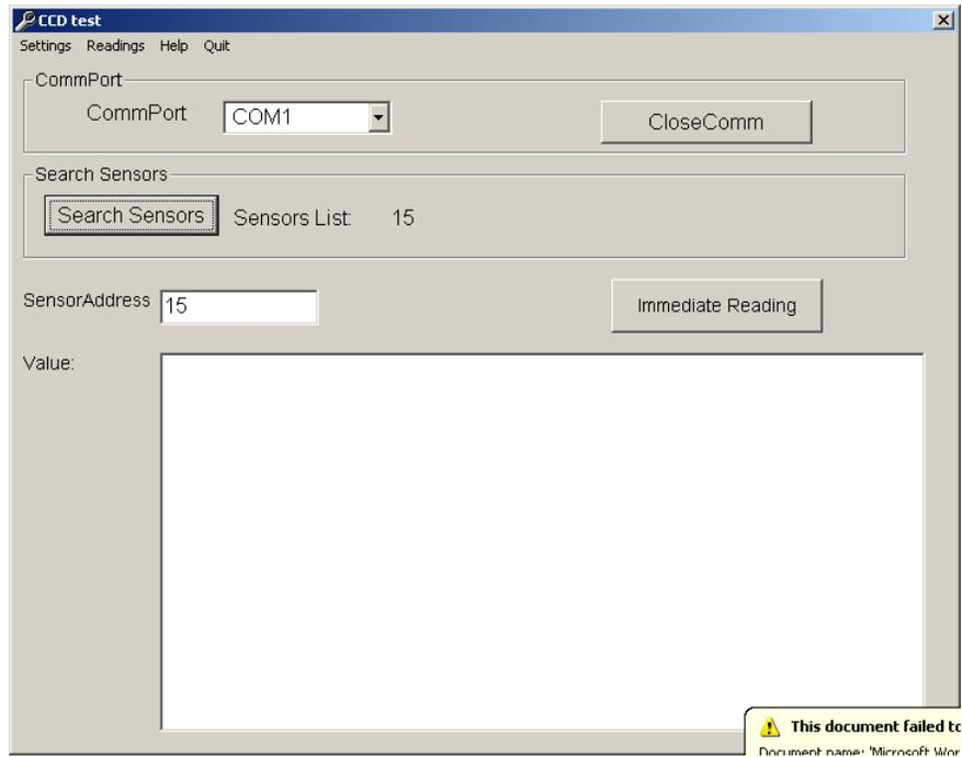
Click **Immediate Reading** to take measurements every 10 seconds from the attached pendulum.
