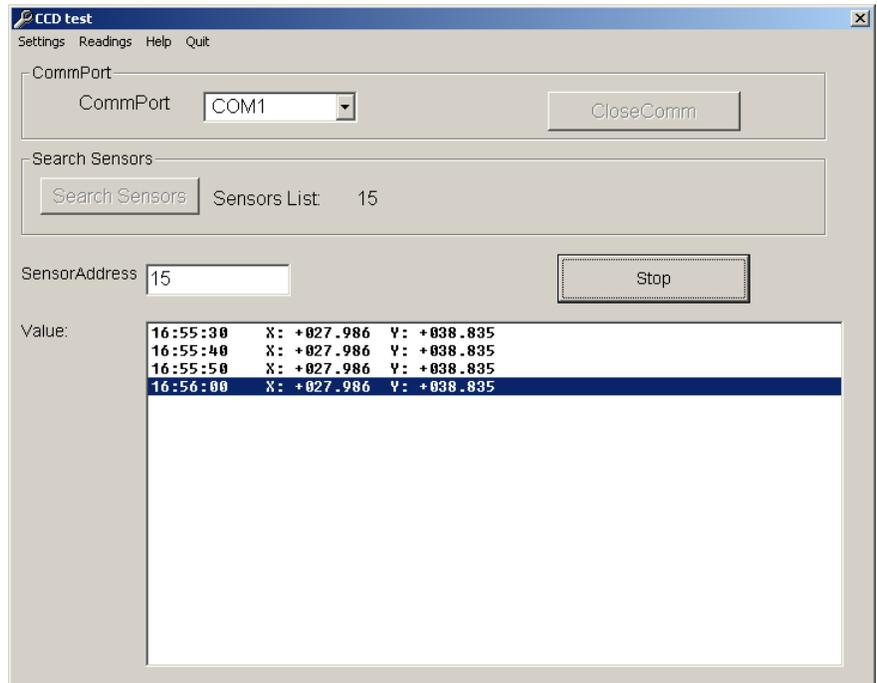
The CCDTest software provides several functions related to the configuration of the pendulum, in particular the setting of the Address, the wire configuration, the setting of the Reference values, the setting of the Clock and the orientation of the outputs. These options are available from the **Settings** menu in the upper left portion of the form.
