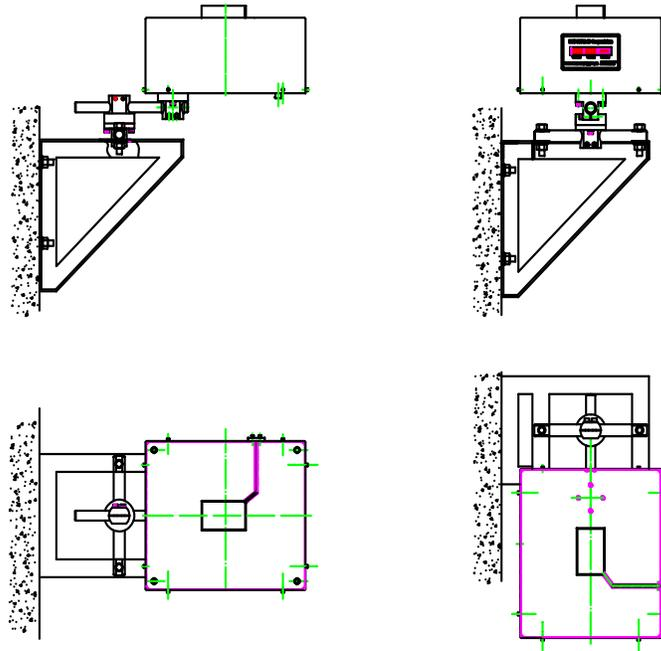
**Figure 14 Universal Bracket mounted on a side wall**
