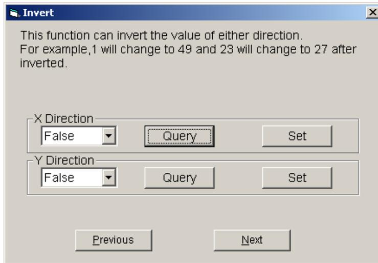
**Note: The Invert options will configure the axis as it is currently displayed. In other words if Swap is True then setting X Direction to True will invert the direction of what was originally the Y axis.**
