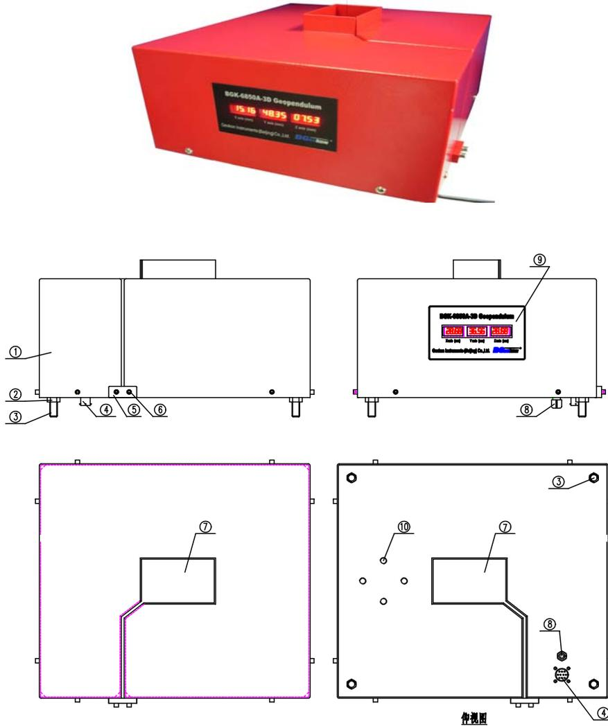
Figure 3. BKG-6850A three-dimensional pendulum system's external shape structure
