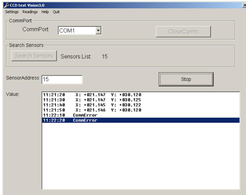
Once the **Sensor Address** is updated the readings should display properly again.
