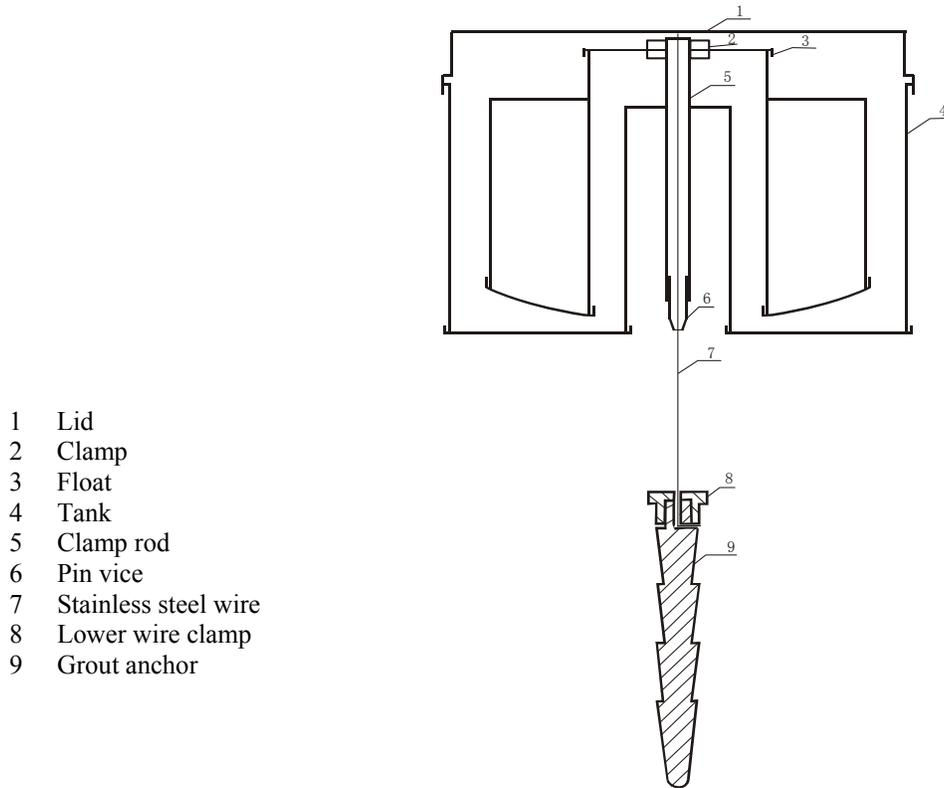
**Figure 9 Inverted Pendulum.**
