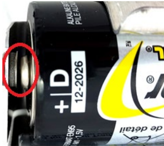
Faulty Battery Installation
