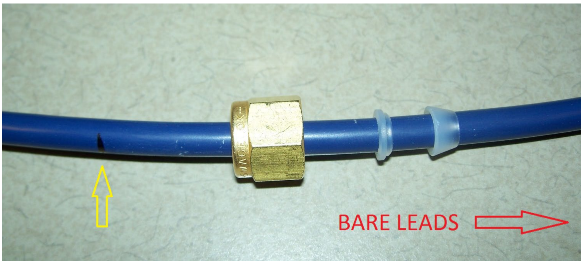
Figure 5 - Swagelok and Ferrule Orientation
