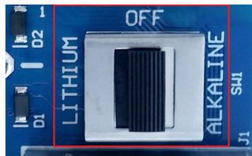
Figure 7 - Battery Select Switch
