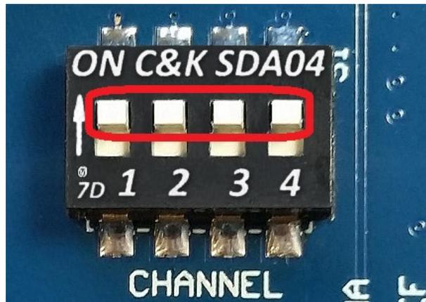
Figure 27 - Channel Selector Switch
