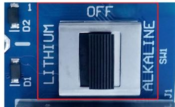
Figure 18 - Battery Select Switch
