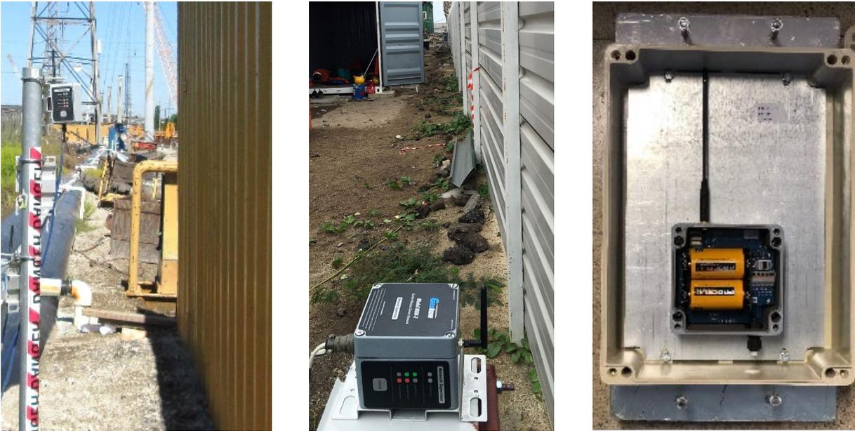
**Figure 4 - Examples of Radio Obstructions**
