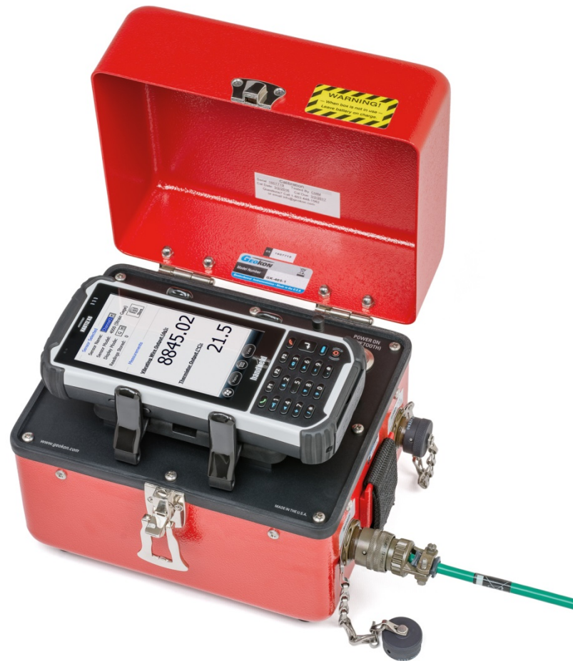
Figure 1 - GK-405 with Handheld PC in Cradle (Shown with the FPC-2)
