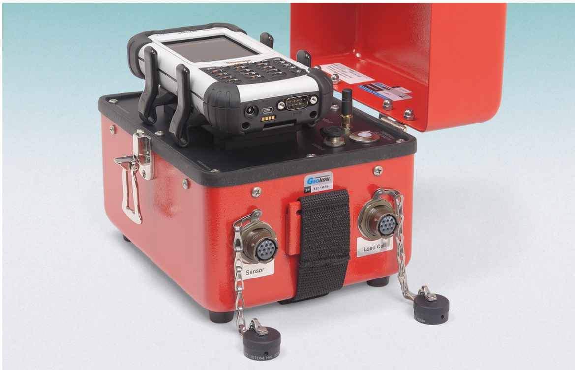
Figure 2 - Vibrating Wire Gage and Load Cell Connectors (Shown with the FPC-1)
