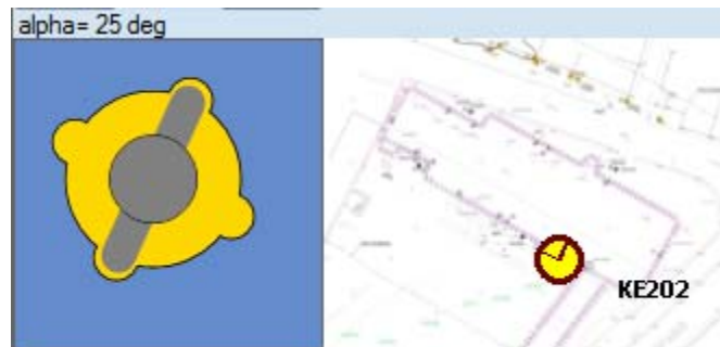
Figure 5.4: Inclinometer probe alignment and key image
