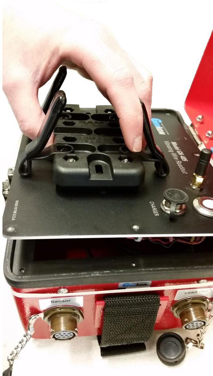
Figure 71 – Removing the Face Plate
