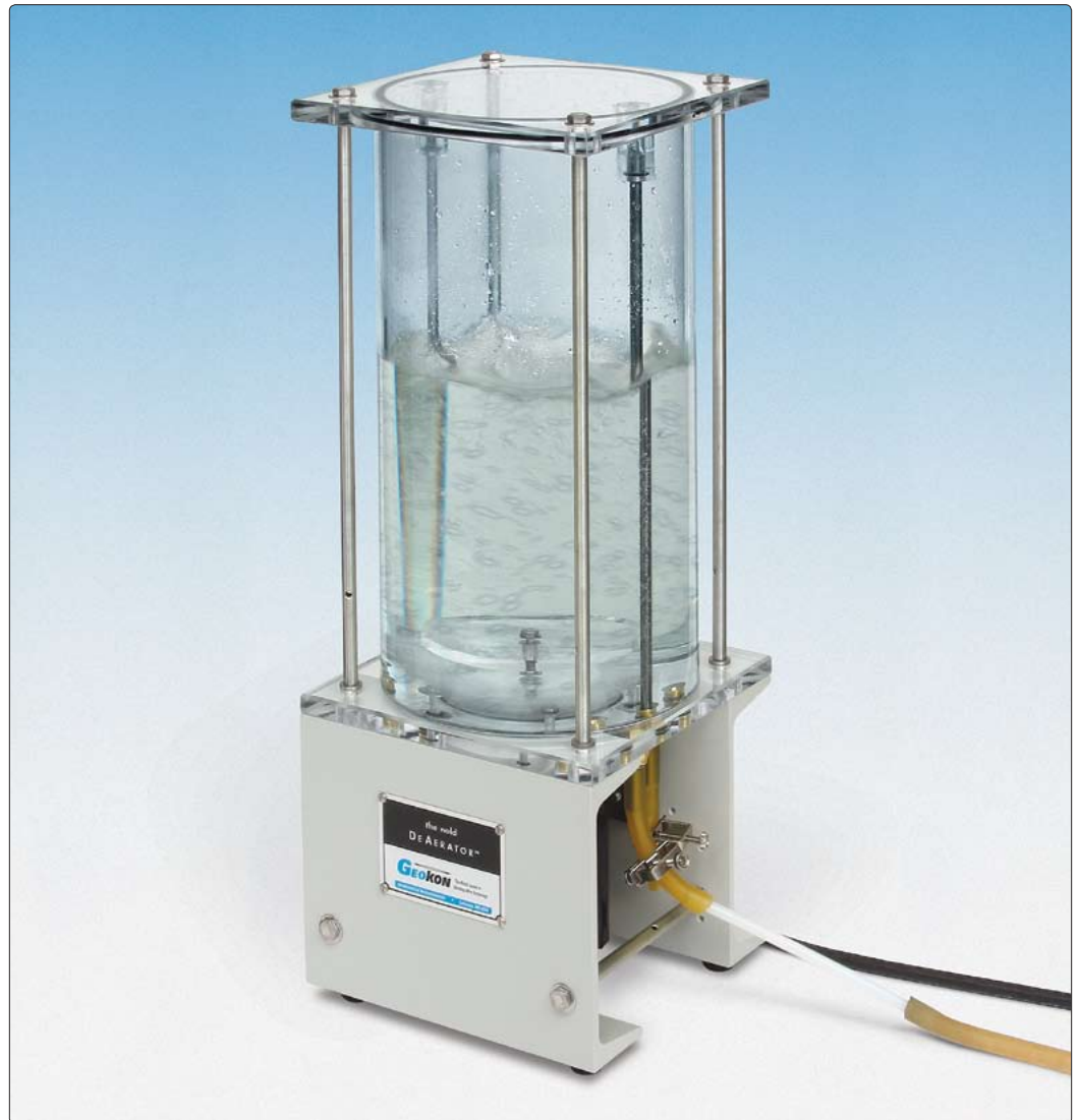
• Model 2100 Nold DeAerator shown degassing a liquid.
