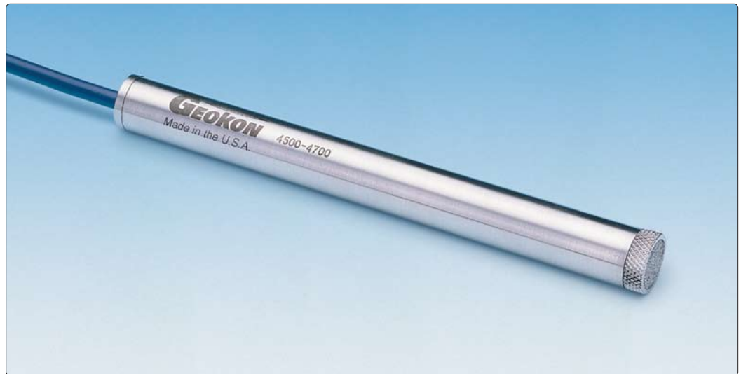
• The Model 4700 incorporated into the Geokon Model 4500 Vibrating Wire Piezometer (Model 4500-4700).
