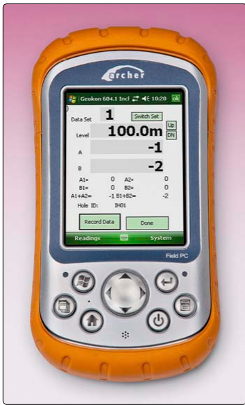
● Model GK-604-6 Field PC showing an inclinometer data reading screen shot.
