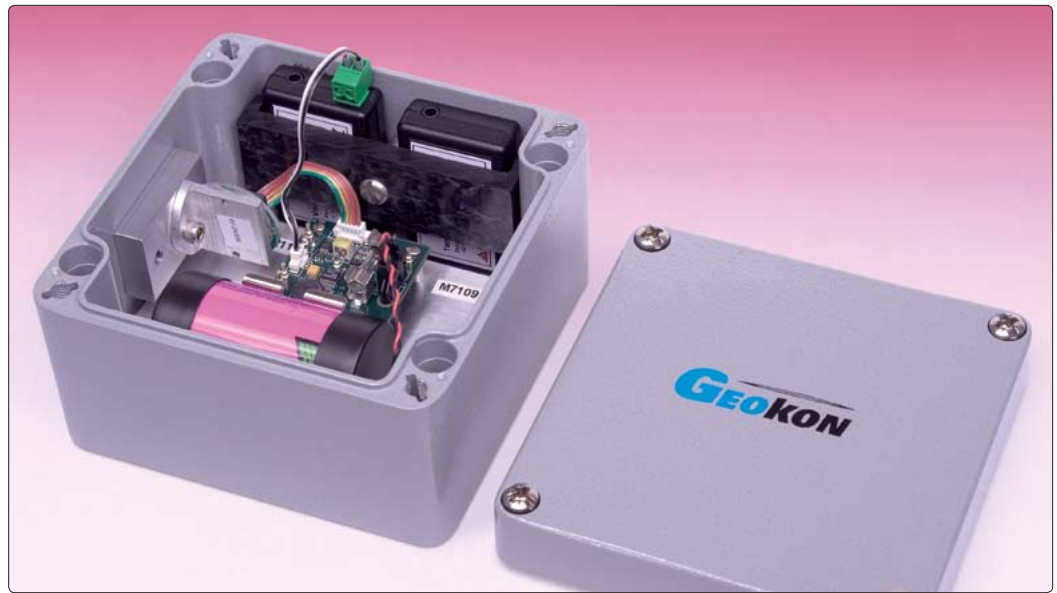
● Model 8101 MEMS Tiltlogger shown with cover removed.
