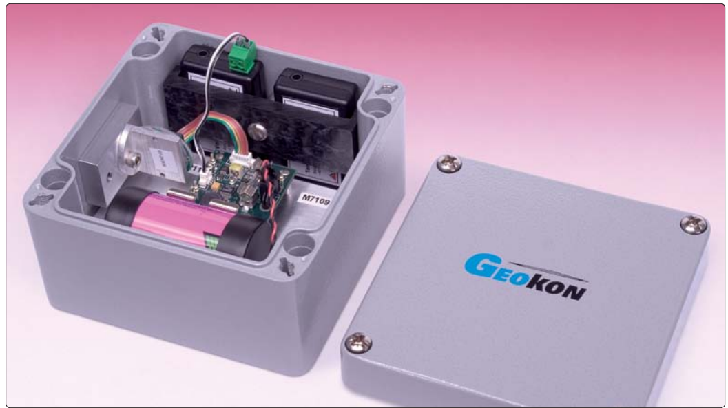
● Model 8101 MEMS Tiltlogger shown with cover removed.
