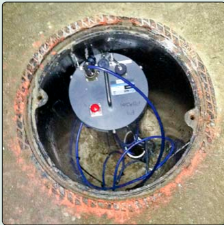
● Model 8040T configured to read a Model 4500 Vibrating Wire Piezometer.
