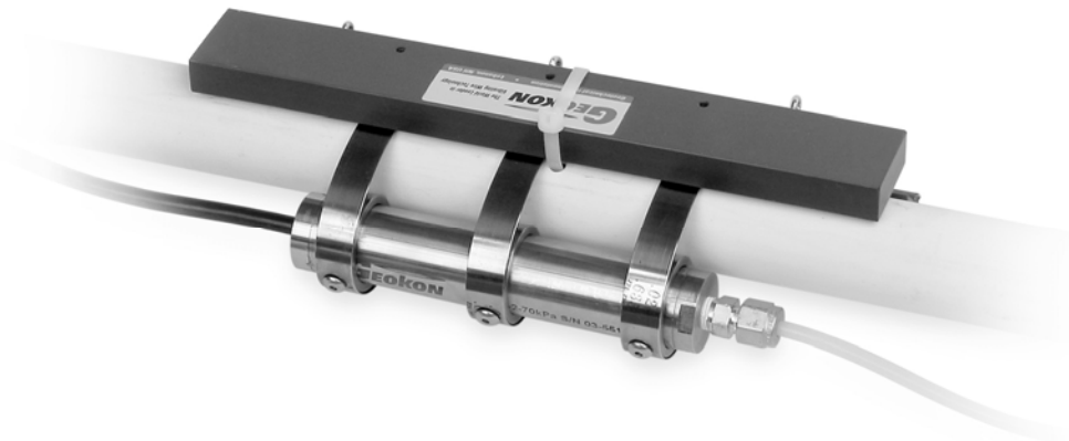
Figure 5 4500MLP Ty-wrapped for Drop Weight Method
