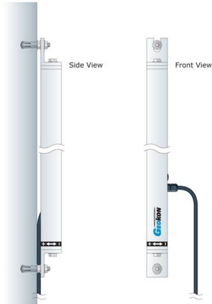
Figure 4. Mounting a vertical beam
