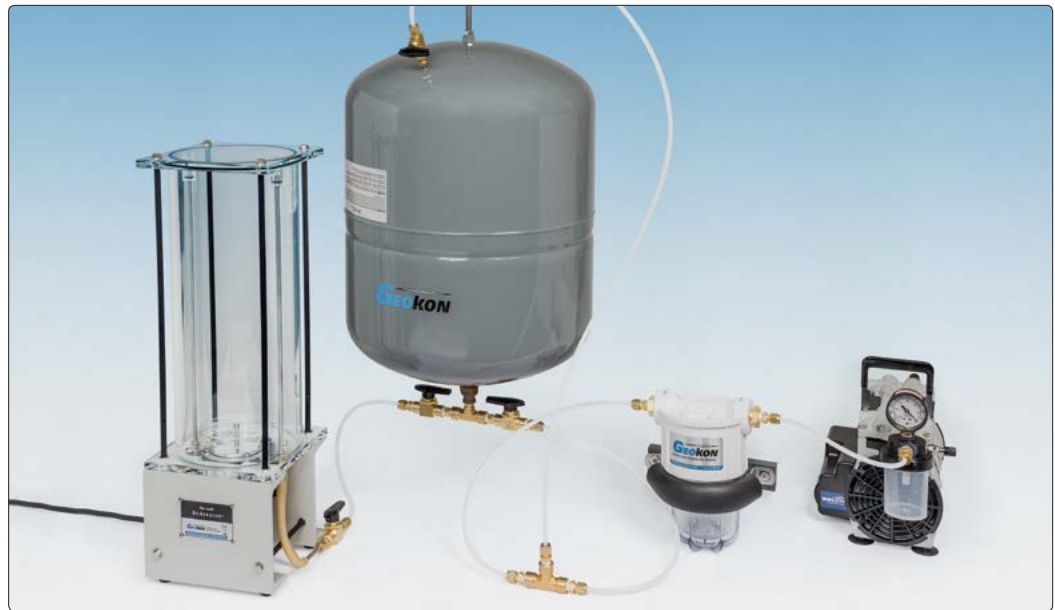
• Typical system components include (from left to right) the Model 2100, a storage tank, a moisture trap and vacuum pump.
