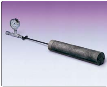
● Model 3200 BPC shown pre-encapsulated in a cylinder of quick setting cement.
