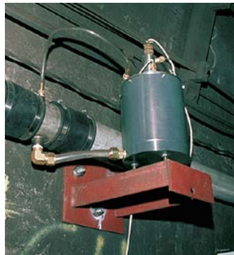
The Model 46750C Liquid Level Vessel with cantilevered mounting bracket.
