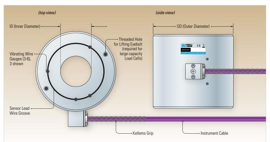
Model 4900 Series Load Cell components.
