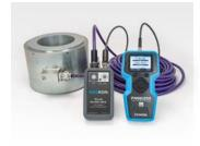
Model GK-406 (Right) utilizing a Model GK-406-MUX (Center) to read a VW Load Cell (Left).
