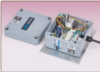
• Model 6161A-2 Biaxial MEMS Tilt Sensor with cover removed.
