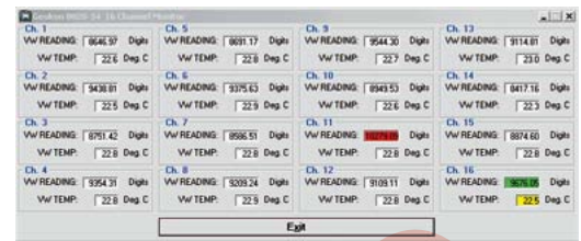
● 16 Channel Monitor screen — green and yellow highlights indicate the current channel being read. The red highlight indicates an over-range condition.
