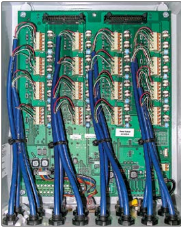
● Model 8032 16 Channel Multiplexer showing internal sensor connections.*
