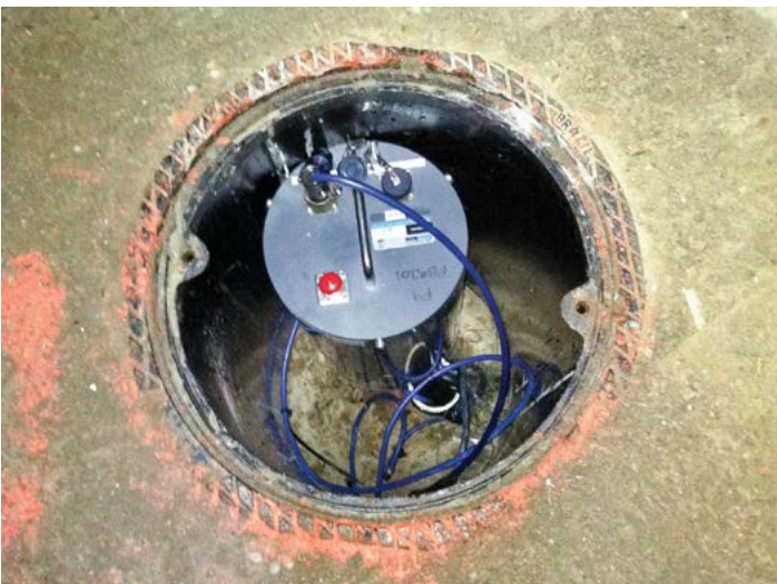
Model 8040T configured to read a Model 4500 Vibrating Wire Piezometer.
