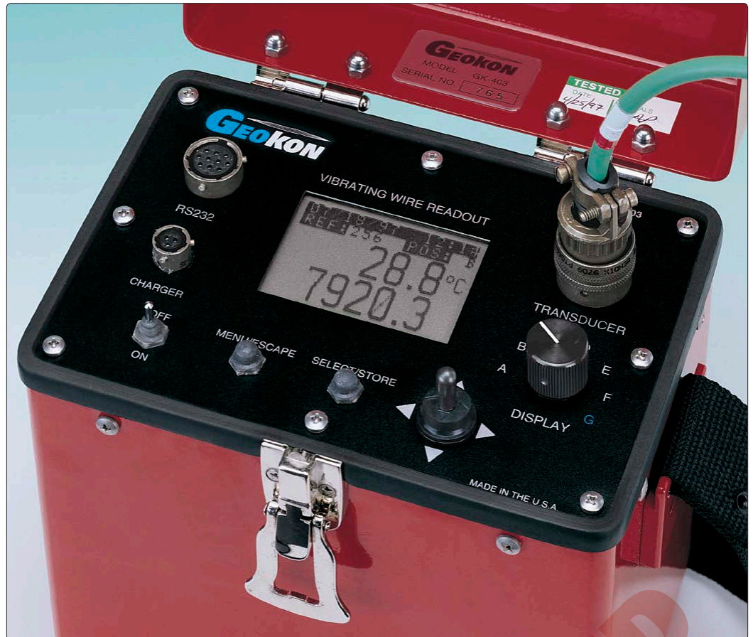
• Close-up of Model GK-403 Vibrating Wire Readout Box control panel.
