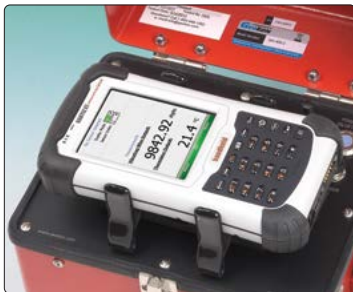
• Live Readings screen shot, displaying vibrating wire strain gauge data.
