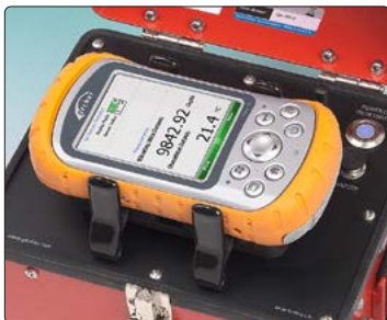
• Model GK-405 VV Readout Dock, shown with the FPC-1 (top) and Archer Field PC (bottom), both of which are compatible.
