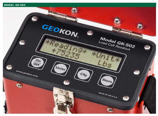
Close-up of the Model GK-502 Load Cell Readout control panel.
