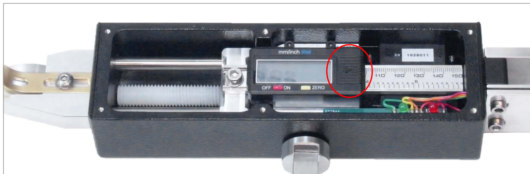
FIGURE 14: Face Plate and Gasket Removed, Digital Gauge Battery Location Shown
