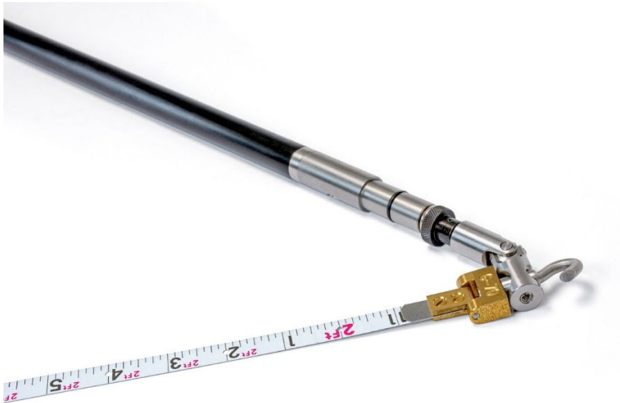
Figure 6 – Hook Manipulator to Tape Extensometer Connection
