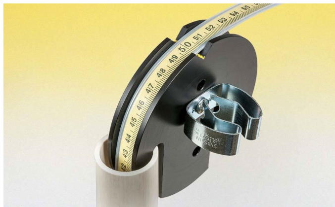
Figure 3 - Tape Guide Mounted to Access Tube
