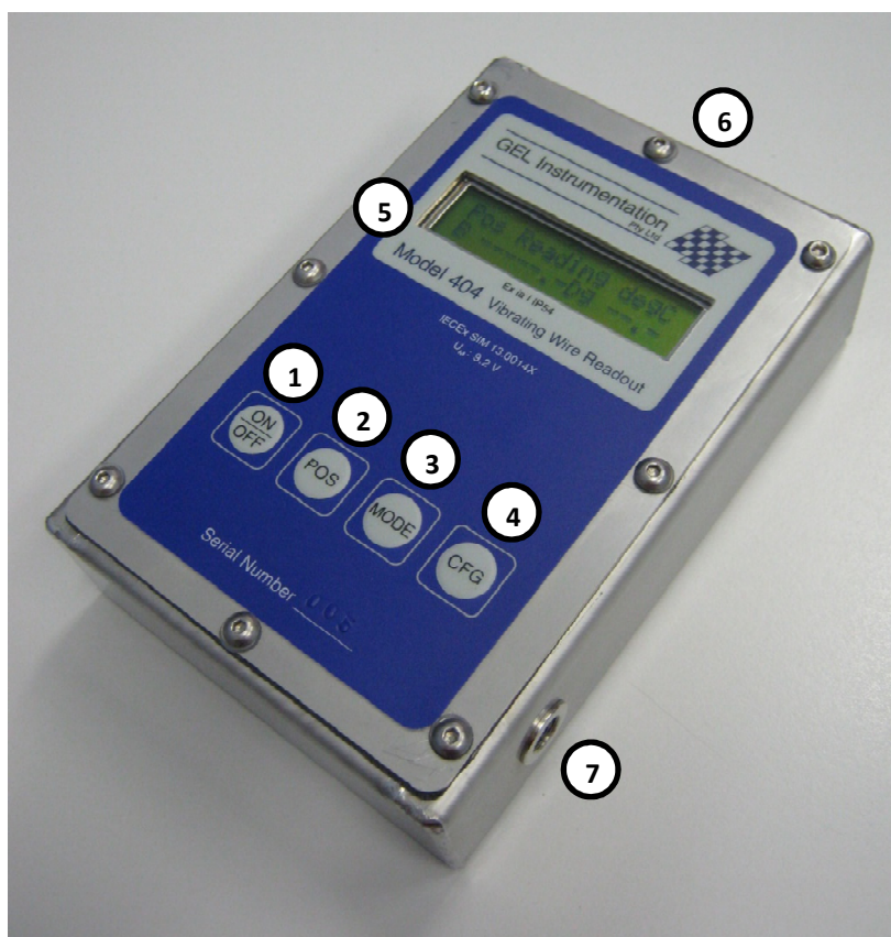
Figure 3 – GEL Instrumentation Model 404 Vibrating Wire Readout (main features)
