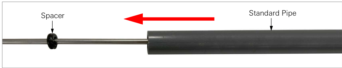
FIGURE 7: Slide Pipe over Connecting Rod
