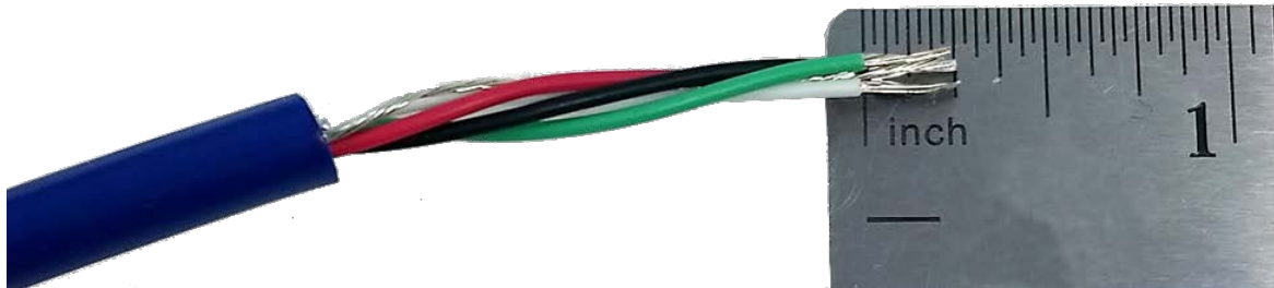
Figure 3 - Cable and Conductor Jackets Stripped Back
