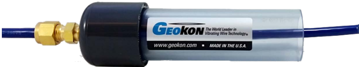
Figure 2 - Initial Cable Insertion
