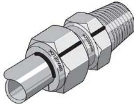
Figure 7 - Marks for Reassembly
