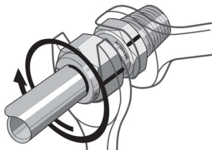
Figure 9 - Tighten Nut Slightly
