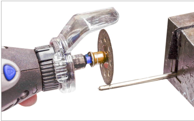
FIGURE 7: Scoring the Sheathing with a Grinder
