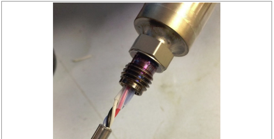
FIGURE 5: Twist and coil the wires to simplify inserting the splice
