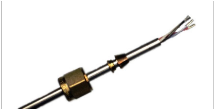
FIGURE 2: Slide the Swagelok nut and ferrules onto the sheathing
