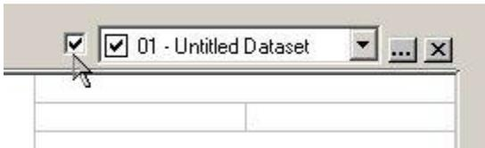
To unload a dataset from the memory, select it from the dropdown list at the top-right corner of the composite graph. Select the **X** button on the right to unload the dataset (see below). Once a dataset is unloaded, it cannot be redisplayed without reloading it using the [Open](#) command from [File Menu](#).
