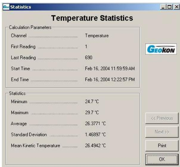
For data recorders with more than one channel, the Next and Previous buttons will be available. This allows the user to quickly view the statistics on each channel. In the example for the RHTemp101, activating the Next button will update the dialog box with the statistics for the humidity channel.
