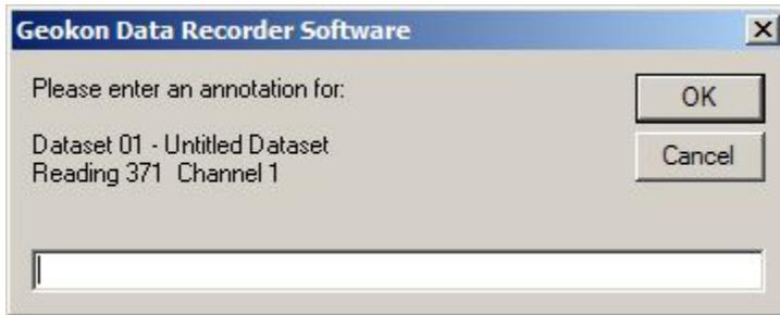
2. Double click the annotate data area on the heading of the graph. Type the annotation in the box as shown below:
