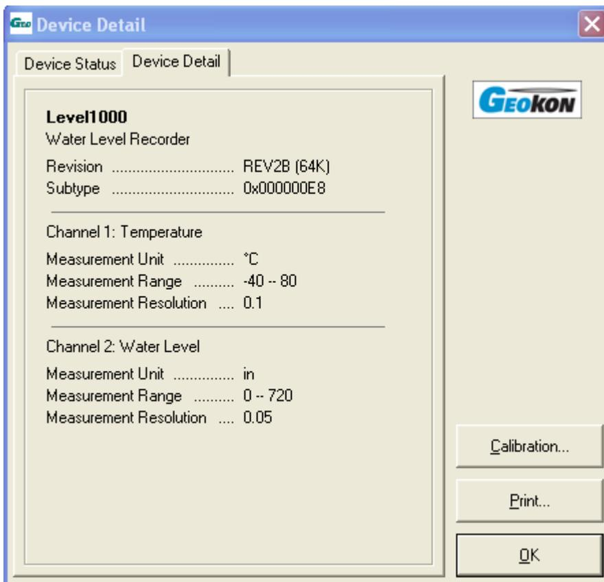
The details include device type (device name as heading), revision number, subtype, and channel information. Information about Engineering Units, Wrap Around, and Calibration will be displayed when the device supports these features.
