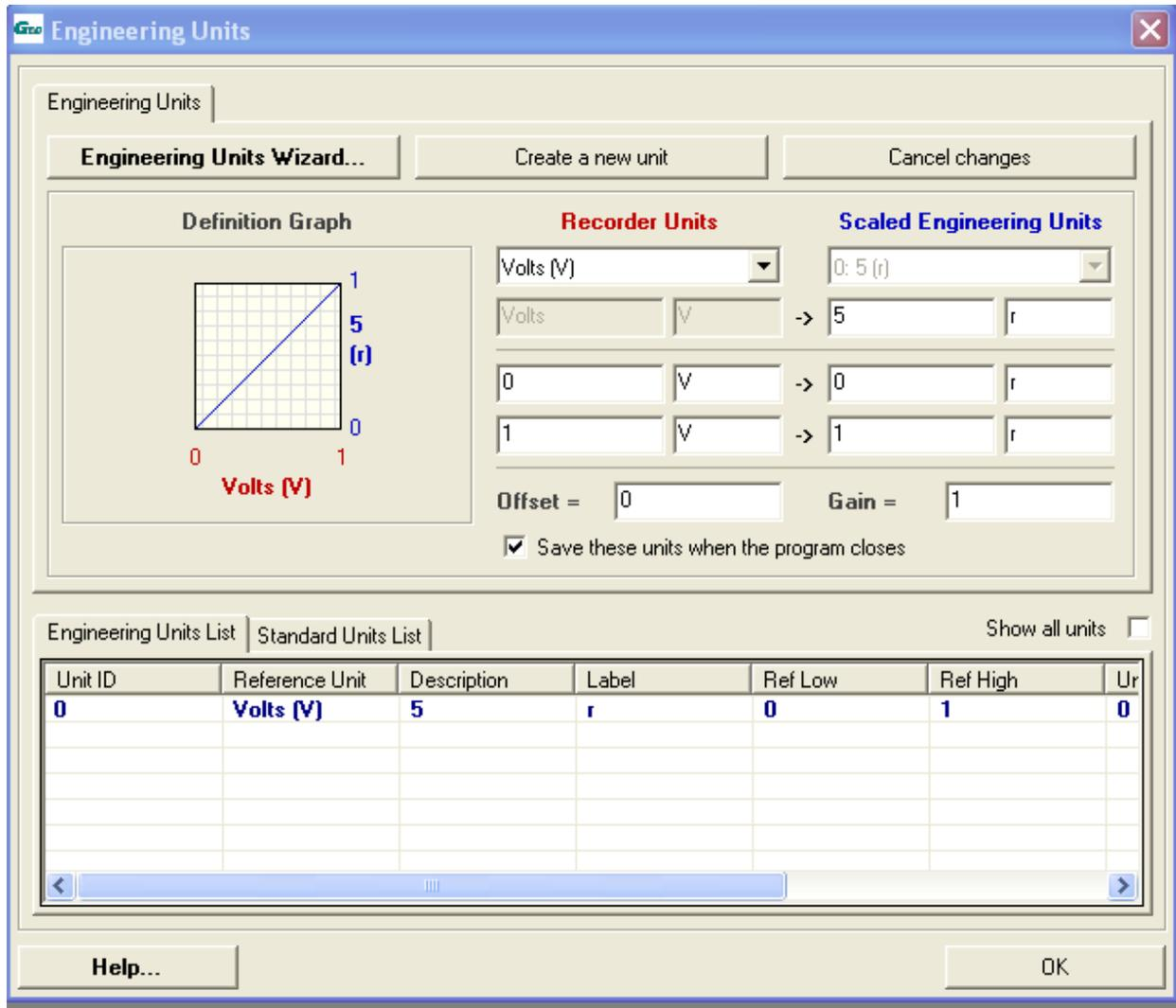
Create **Engineering Units** by using the **Engineering Units Wizard** button or **Create a new unit** button on bar below.
