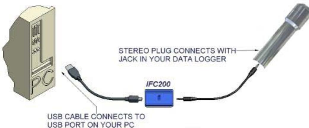
1. Insert the male connector of the IFC200 interface cable into the female receptacle of the data logger. Insert the female USB connector into the USB.
