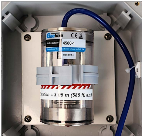
FIGURE 6: Sensor and Sensor Cable Secured
