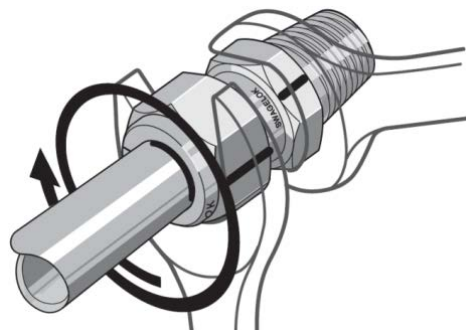
Figure 18 - Tighten Nut Slightly
