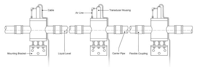
Figure 2 - 4675OC – In-Line System
