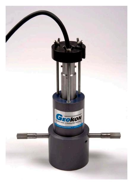
Figure 16 BDG Calibration Rig
