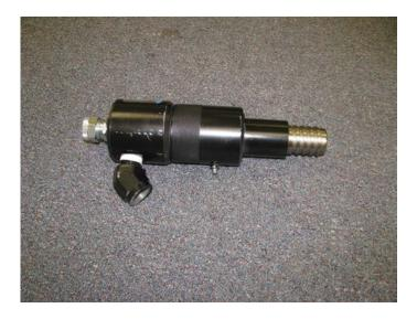
Figure 1 Modified Water Swivel
