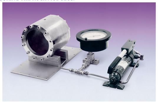
Figure 7 Biaxial Modulus Chamber with Pressure Gage and Hand Pump
