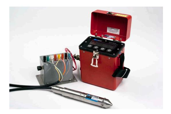
Figure 3 Model GK502 Readout Box
