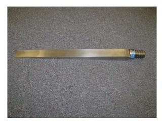
Figure 4 Core Breaker Wedge
