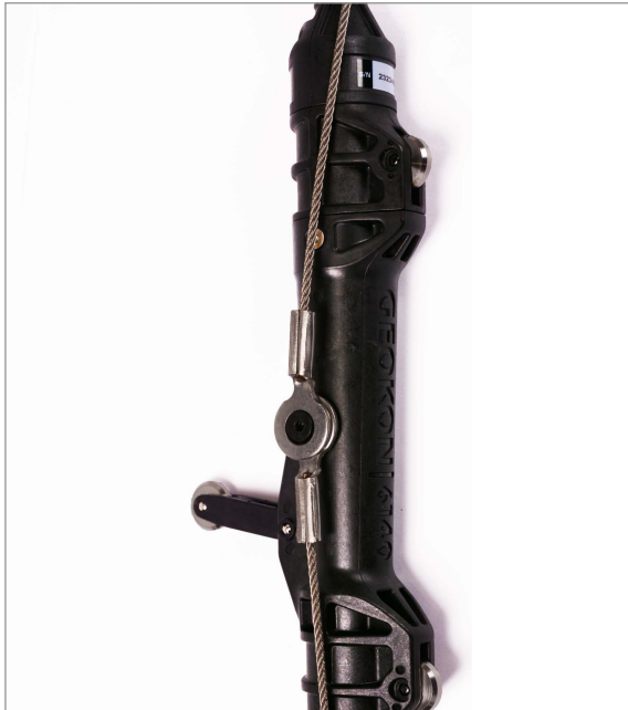
FIGURE 11: Arrange Eyelet from the Next String Section Over Existing Eyelet
